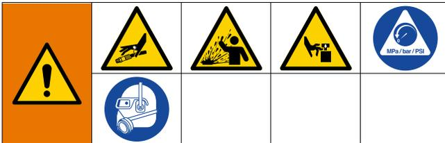
This equipment stays pressurized until pressure is manually relieved. To help prevent serious injury from pressurized fluid, such as skin injection, splashing fluid and moving parts, follow the Pressure Relief Procedure when you stop spraying and before cleaning, checking, or servicing equipment.
